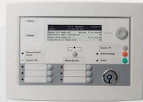
The floor repeater terminals and displays FT2010 and FT2011 display system status and events at floor level. They enhance user convenience, as visibility can be configured individually. Floor repeater terminals and displays are connected directly on the C-NET loop, saving cabling and installation costs. And FT2010 and FT2011 enhance safety because they remain functional even in case of an open or short circuit.
